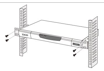
4.After the brackets are attached to the device, use suitable screws (not provided) to secure the brackets to the rack, as illustrated in the following figure.
