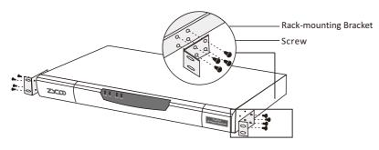
3.Install IP PBX to the right place in the rack, and then attach the brackets to the device.
