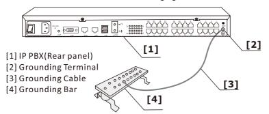
If the device is installed in the normal environment, the device can be grounded via the PE (Protecting Earth) cable of the AC power supply as shown in the following figure.
